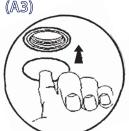
Fit the 'Plastering' cardboard disk into the housing.
