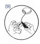
Connect LED Driver or Light Engine to 230V lighting circuit then fit into the ceiling housing.
