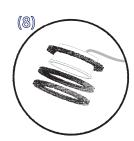
Fit Magnetic Rings onto Light Engine Note: 3 Rings required with at least 1 ring behind.
