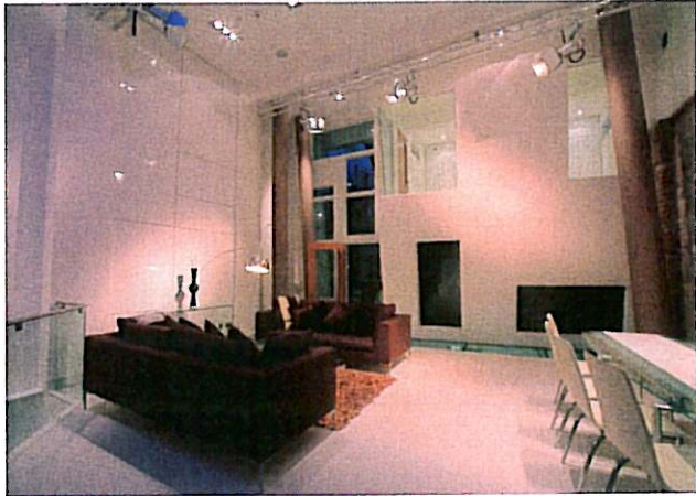
High level spots on a gantry – and high output recessed fittings – evoke the building's earlier role. Leax 24-circuit dimming racks are controlled by four scene-setting wall plates.
