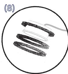
Fit Magnetic Rings onto Light Engine
